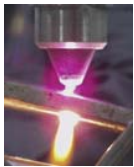
Fig. 1 Drilling using high energetic electrical plasma [1]
