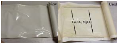
Figure 1. Comparison between new and used membrane
