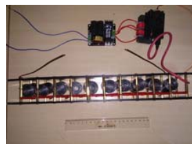
Fig. 4 Combination of Marx Generator and ZVS as pulse generator
