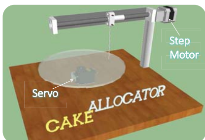
Fig. 1 3D model of the cake allocator
