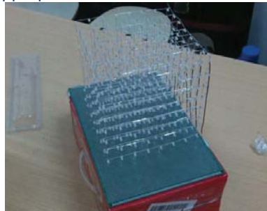
Fig. 2 The whole structure of the CUBE8
